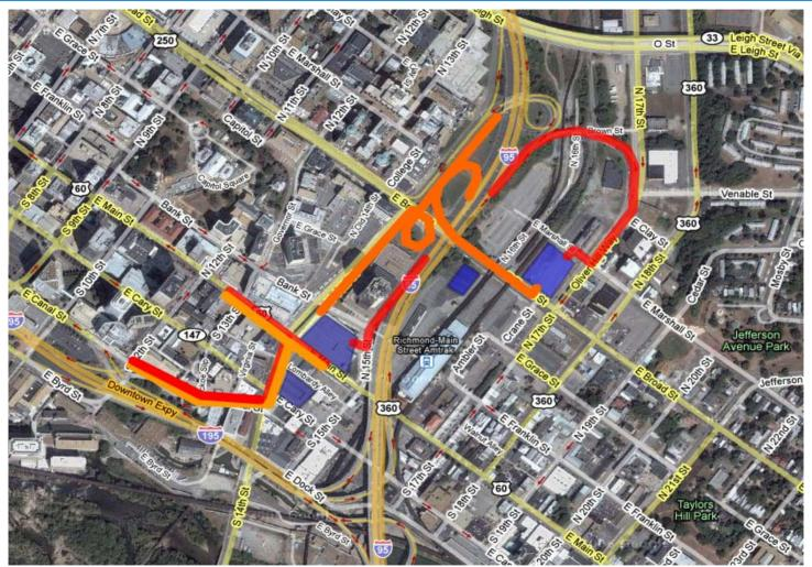
Red Lines show traffic ingress into decks, shaded in blue Orange lines show traffic egress from decks
