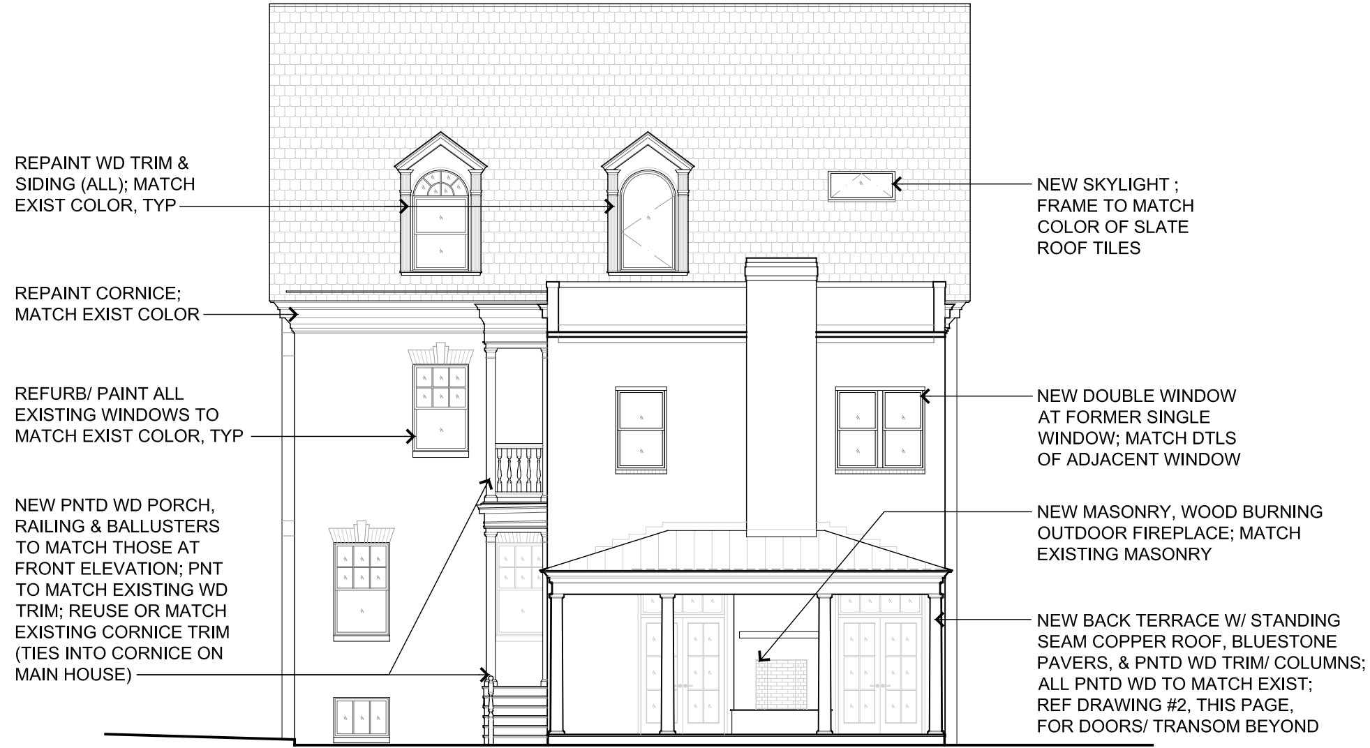
1 NORTH/ REAR ELEVATION - PROPOSED 1/8" = 1'-0"
